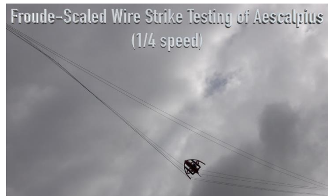
Figure 23.6.4 Froude-Scaled Wire Strike Flight Testing of Open-Rotor, Closed-Rotor and Asklepios Drones
