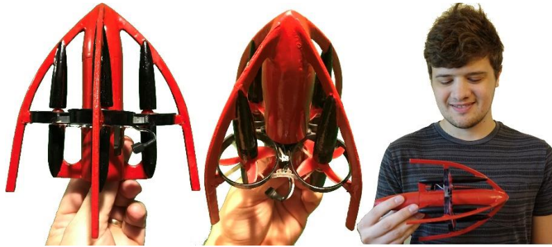
Figure 23.2.6: 1/27th Scale Asklepios Wind Tunnel and Flight Test Aircraft
