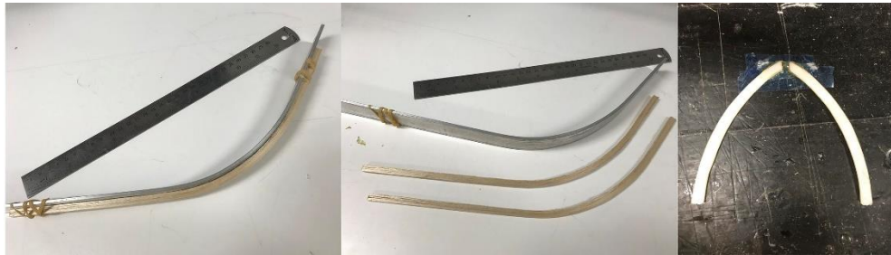
Figure 23.2.3: Formation of Balsa-Kevlar Arch Assembly
