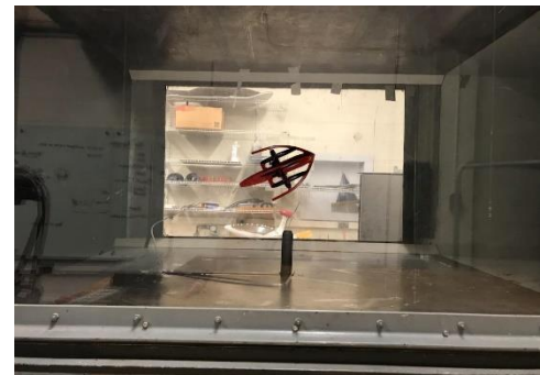
Figure 23.3.1: Test Aircraft Mounted in the University of Kansas 3 x 4' Subsonic Tunnel
