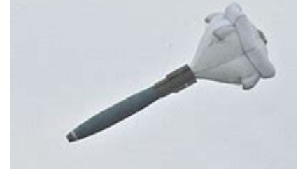
Figure 13.1: Example of a MK82 Bomb with a Ballute
