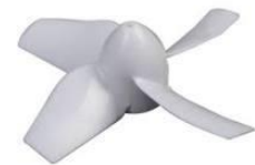
Figure 23.2.2: Injection-Molded Nylon 40mm Rotor for Test Aircraft
