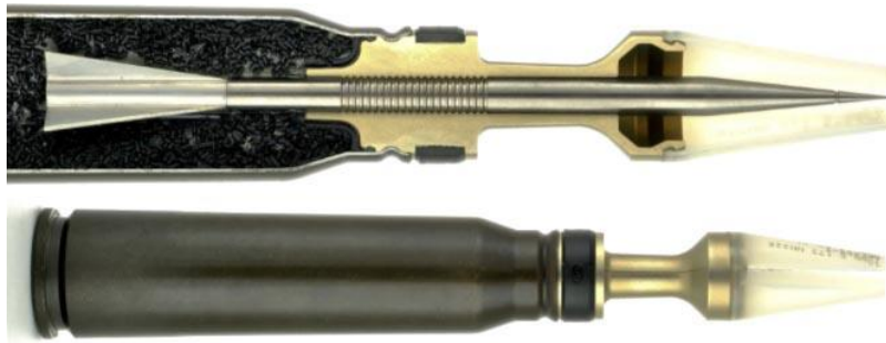
Figure 11: Typical Navy 30mm Saboted Ammunition 30x173 NM225 APFSDS-T [30]
