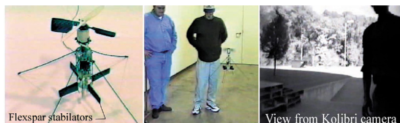
Figure 1. The Lutronix Kolibri, the world’s first VTOL MAV enabled by piezoelectric flexspar stabilizers (1997) [11].
