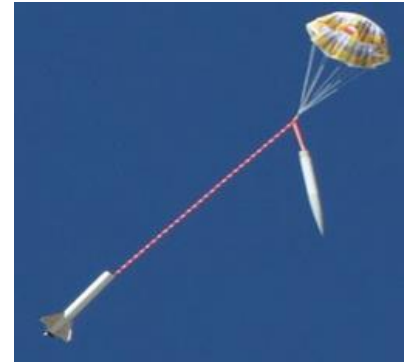
Figure 7.11: Emergency Parachute Deployment [47]
