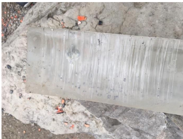
Figure 8.18 Wad of Kevlar Strands Embedded Within Target
