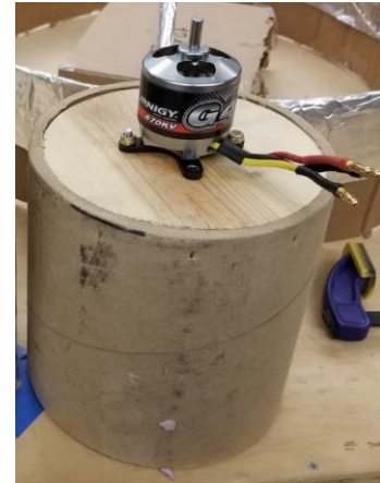
Figure 12.6: Mounted Turnigy 270KV Motor (Same as Specified for Design)
