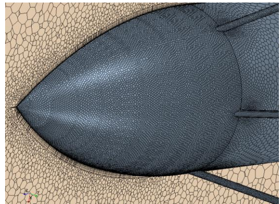
Figure 11.6: Surface Mesh and Prism Layers at Nosecone
