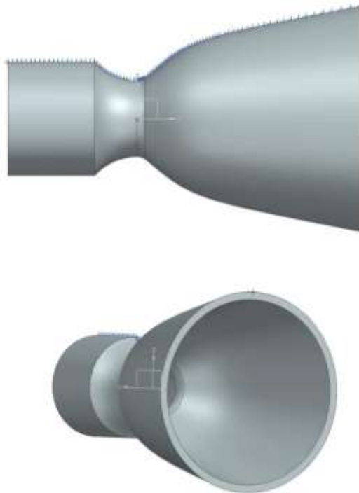
Figure 4.1: Theoretical Nozzle Design for the 105mm RAIDER
