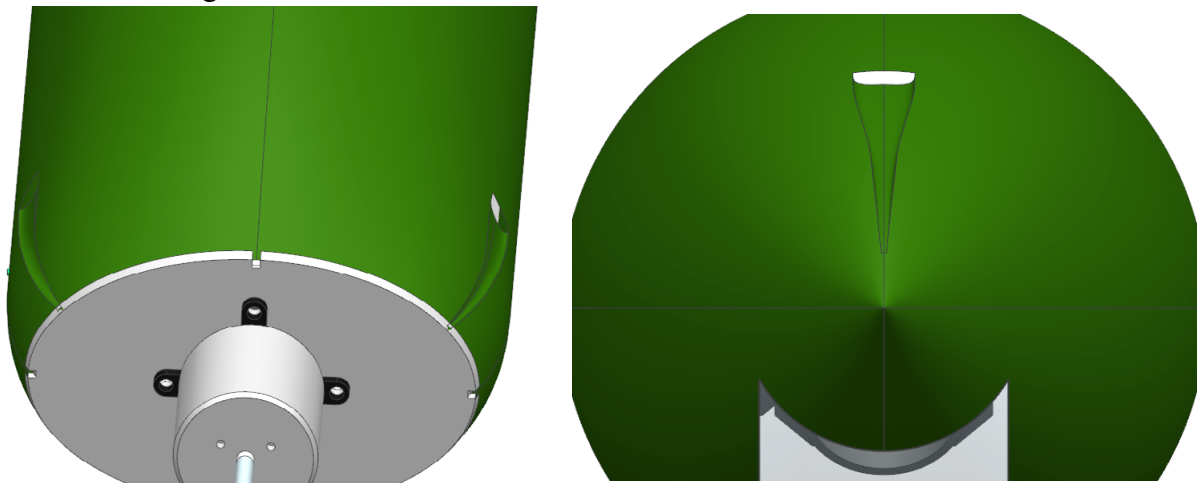
Fig. 20.9: Fuselage and Sensor Pod NACA Inlets (NTS)
