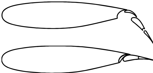
Figure 11.5.1 Flap setting at wing root extended and retracted
