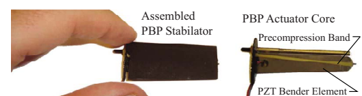
Fig. 21 PBP actuated flight control surface for micro aerial vehicle [41]
