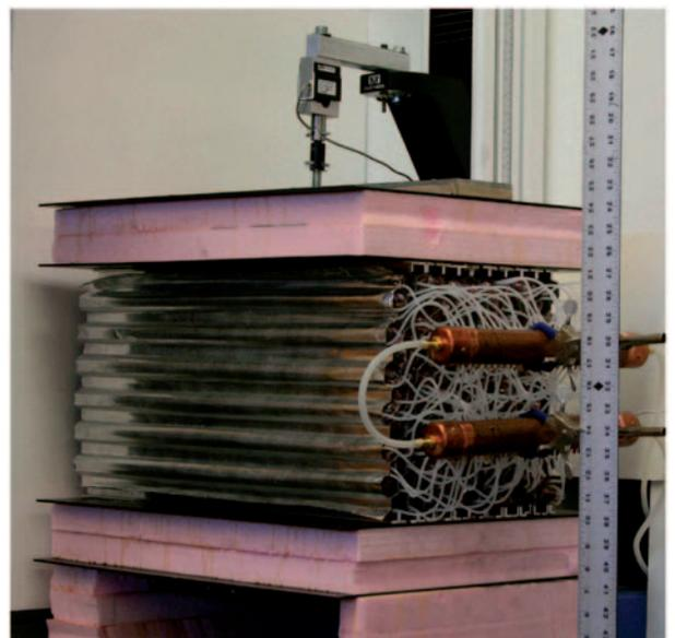
**Figure 8.** Experimental test setup of pressurized flexible-wall honeycomb in Instron 3345 (longitudinal compression).
