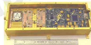
High-Efficiency L-band T/R module to be modified with integrated calibrator
