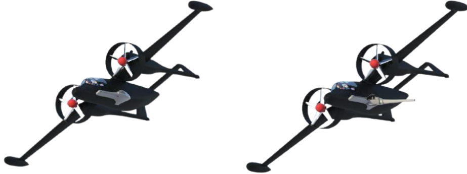
Fig. 15 Example Ground Attack Aircraft Designed to Loft and Fire HBASS Rounds with Strafing Fire (L) and Direct Orbiting Fire (R)
