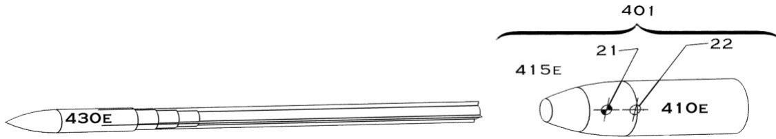
Fig. 5 One Species of Ballistic Aeromechanically Stable Sabot (BASS) Flechette and Sabot [10] [11]
