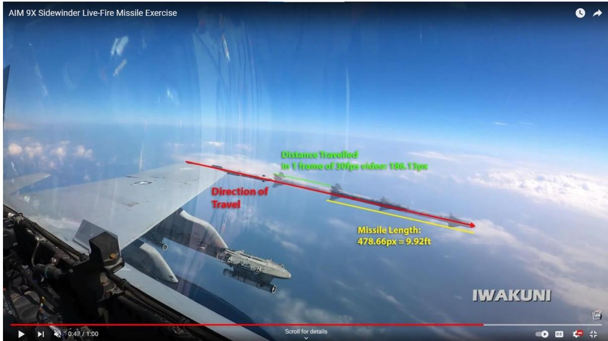
**Figure A.1: Off-Rail Speed Calculation Screenshot (Ref. 3)**
