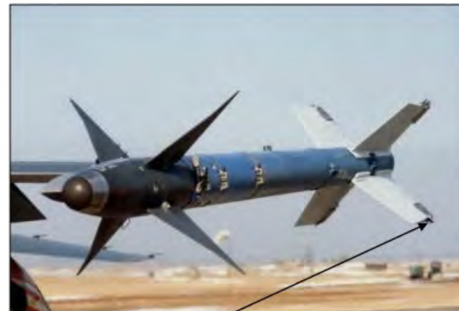
AIM-9M: Rollerons ( ~ 30,000 rpm )
