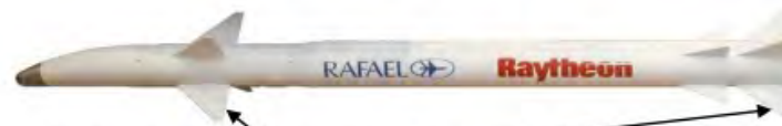
Stunner: Blended Canard – Tail Control Provides Direct Lift Divert Accuracy and Skid-to-Turn Maneuverability.
