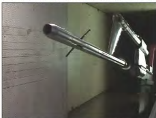
Video of DAGR Free-to-Roll Tail Stabilizers )
