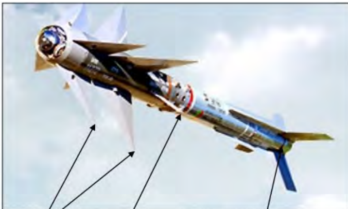
Python 4: Split Canards, Dedicated Roll Control, Free-to-Roll Tail Stabilizers
