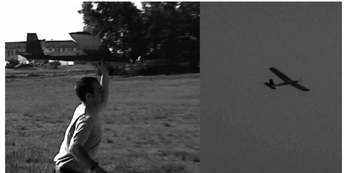
Figure 8. Gentle Lady type 6-6ft (2m) UAV VSS test aircraft type during launch and in free flight.
