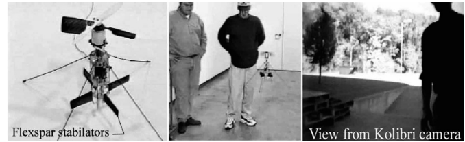
Figure 1. The Lutronix Kolibri, the world's first VTOL MAV enabled by piezoelectric flexspar stabilators (1997).
