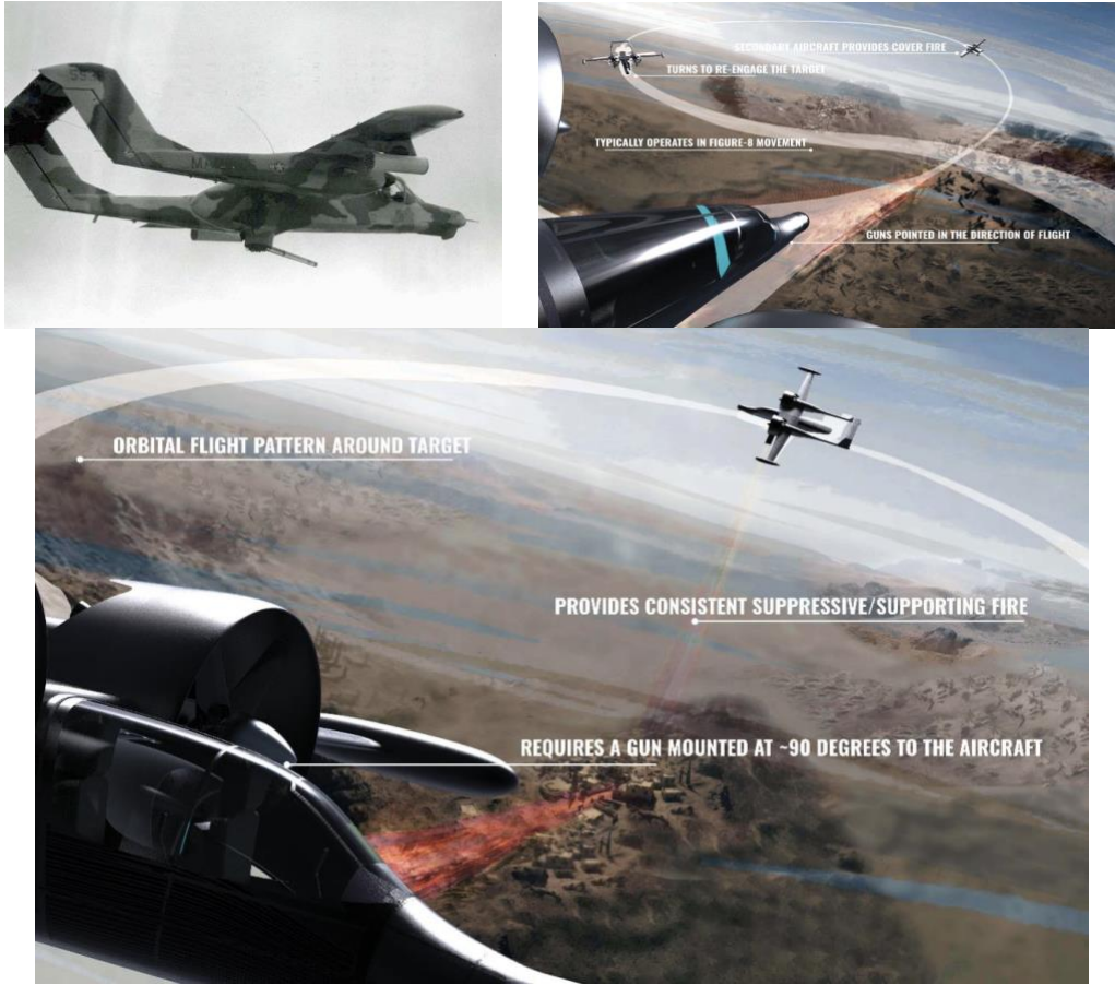
Fig. 16 OV-10 Bronco with Ball Turret M197 20mm 3 Barrel Gatling Gun, Conventional Figure-8 Type Target Engagement and Orbiting Fire Possibilities
