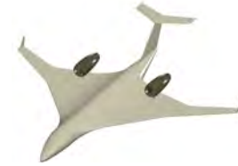
Figure 8.1.1 Blended Wing Body
