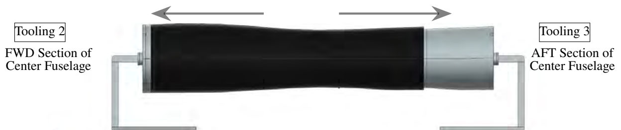
Figure 14.3.1 Removing Process for Center Section of Fuselage Tooling
