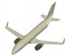
Figure 8.1.6 Low Wing L-Tail
