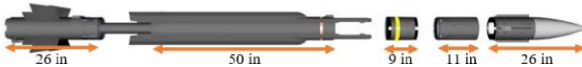
Figure 4-1: Propellant volume estimation of the MICA missile [27]
